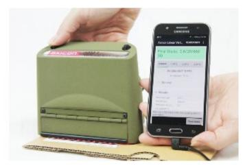
Barcode-Test has an all in one, out of the box, Axicon linear barcode verifier connected to Samsung Galaxy J3 smartphone using the Axicon Android software. Choose from the Axicon 6000, 6500 or 7000 series verifiers.
